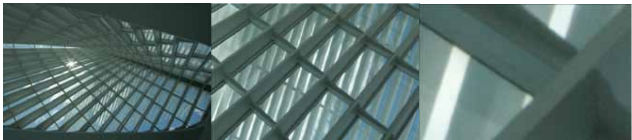
Figure 3 shows the same image at three levels of magnification. On the left 'A' is full size; in the center 'B' is 1:1; and on the right 'C' is 8:1. In both A and B the edges of the stainless steel ceiling beams are crisp as you would expect. On the right in C the edges of the beams are soft which is an artifact of the analog to digital conversion process, and why sharpening is an essential part of the digital image-optimization process.
